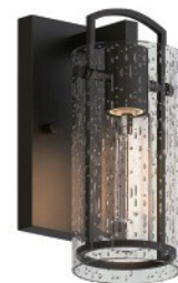
Wall Mount: TH2023-021-1W Size: W4.5" E5.5" H10" Finish: Matte Black Material: Steel+Clear Glass Wattage: 1-E26
